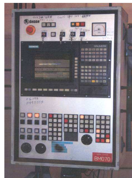
Control Panel Siemens
